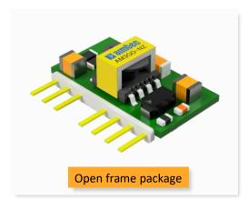
The AM3GO-NZ series is a high-performance open frame DC/DC converter specifically designed for a variety of telecom applications. It features 3W of output power with no requirement for minimum load, a wide input voltage of 36-75VDC, operating temperature up to 85°C and tested I/O isolation of 1500VDC.
